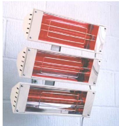
Model No – HLX45 (Consists of 3x HLX15 + 1 x HLB3 Bracket) Each fitting is 220/240v 1500w 6.25amps
